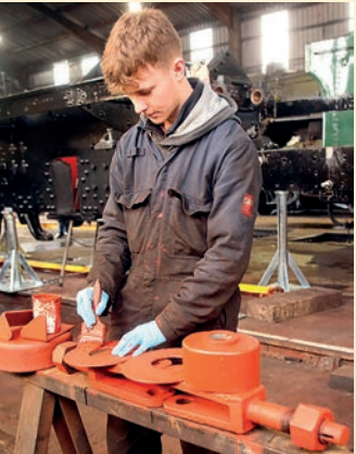
Apprentice Jacob Cox applying protective layers of paint to the loco's components
